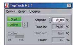
Each laboratory instrument has its own control window
