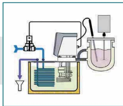
ME, HE and SE circulators can also be equipped with an automatic cooling water supply. As these instruments do not have an integrated solenoid valve controller, they require:
