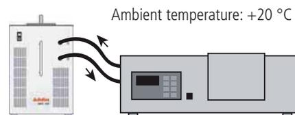
**AWC100 is designed to cool water in closed loops. The unit permanently removes heat from water as it flows through the machine.**
