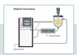
The Mag Drive Booster Pump can increase your fluid pressure up to 2.1 bar. The stainless steel design of the pump provides excellent resistivity against chemical effects. The magnetically driven design guarantees 100 % leakage free operation over an extraordinary temperature range of -90 °C ... +250 °C.
