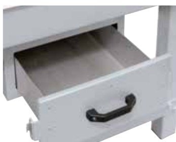
Drawer for collection of liquid wax
