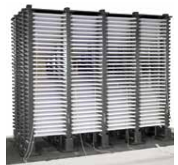
Kiln furniture for small ceramics components
