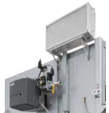
Direct gas-firing at a chamber dryer
