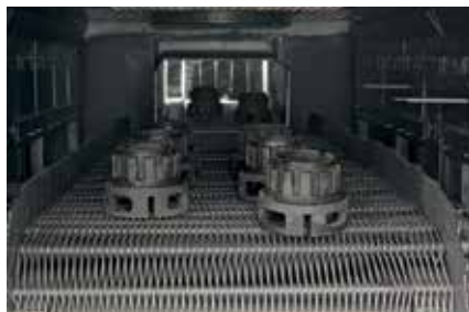
Mesh belt drive in a continuous furnace
