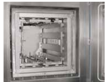
Tungsten heating chamber
