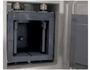
Graphite heating chamber
