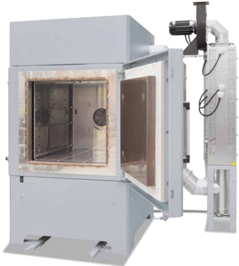
Air circulation chamber furnace NA 500/35 DB200 for debinding in air with catalytic afterburner system
