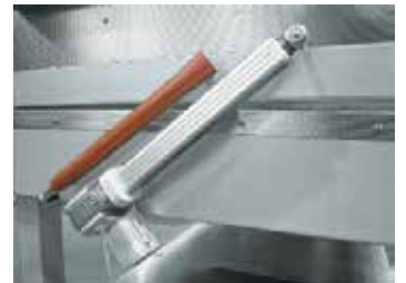
Automatic lid opening via electromechanical spindle
