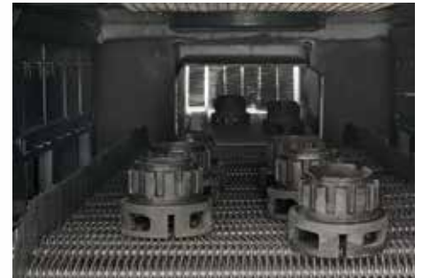
Mesh belt drive in a continuous furnace
