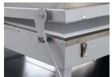
Locking device provides for defined lid opening in different positions and accelerated cooling
