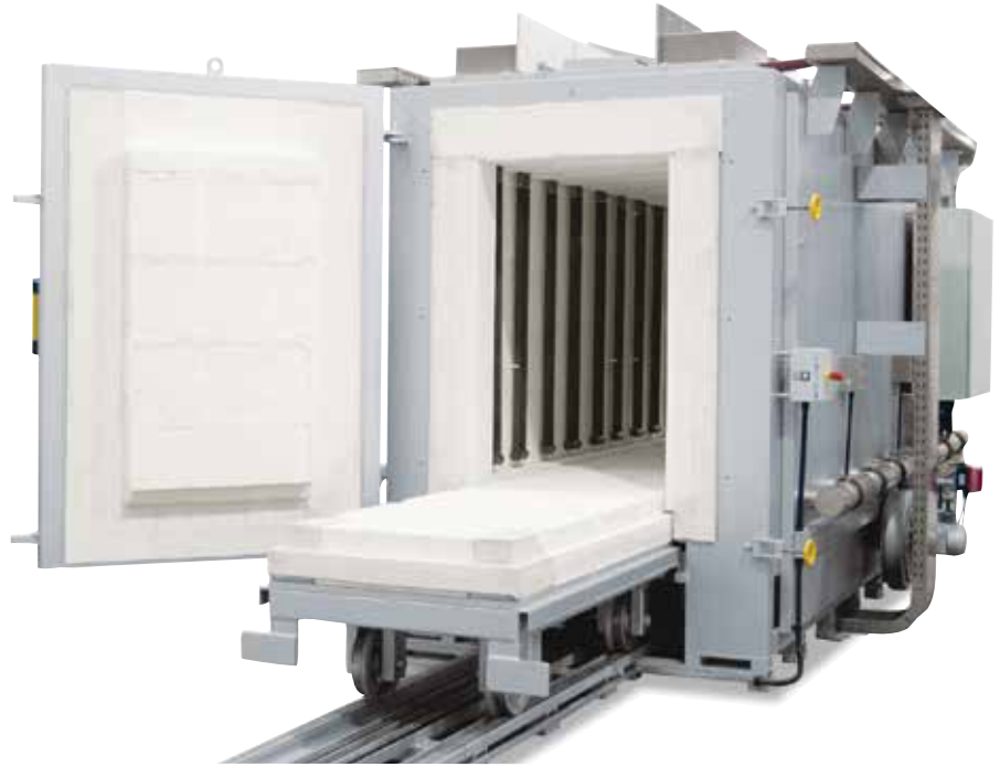
WHTC 4000/15 with bogie on rails and fan cooling
