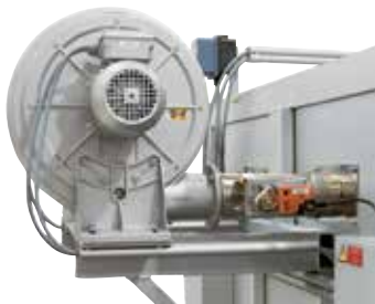
Cooling fan for accelerated cooling
