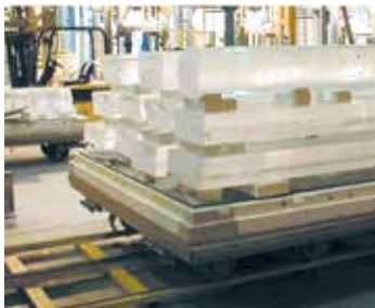
Bogie hearth furnace for tempering quartz rods
