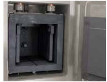
Graphite heating chamber
