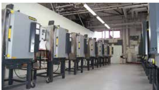
Chamber kiln N 200 for tempering
