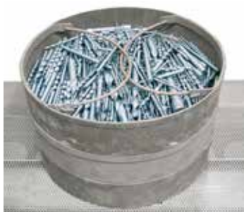
Bluing of drills in water steam atmosphere in a furnace of the NRA range
