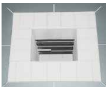
Two-Side heating with SiC rods
