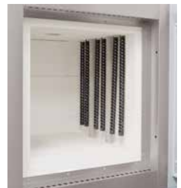
Vertically mounted SiC rods
