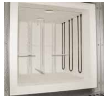
Fresh air injection through perforated injection tubes
