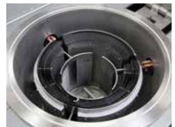
Cylindrical retort with tungsten heating
