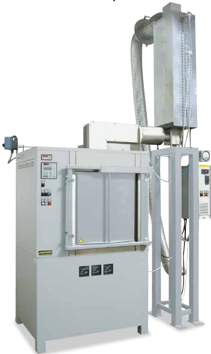
HT 160/17 with catalytic afterburning system
