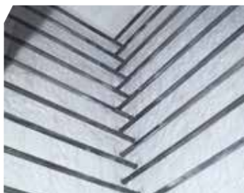
Heating from 4 sides with SiC rods
