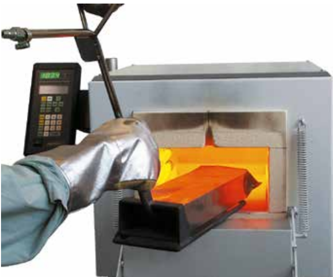
Hardening in annealing tray with alloy bag
