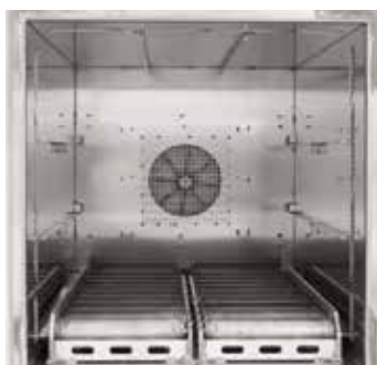
Roller conveyor in furnace N 250/85HA
