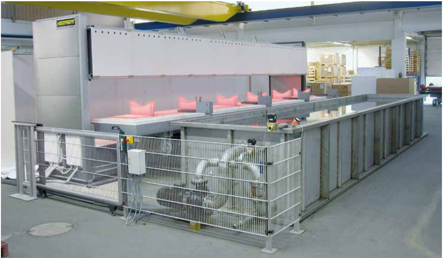
Tempering plant with light-top furnace H 4263/12S and water bath
