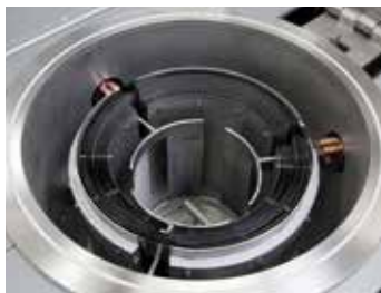
Cylindrical retort with tungsten heating
