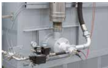
Gas burner positioned along the furnace side
