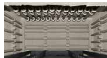
Furnace chamber with optional heating elements in the ceiling when used for preheating of sheetmetal plates
