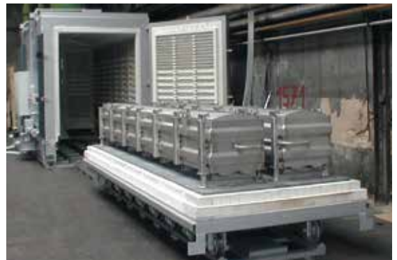
Bogie hearth furnace with gas supply system
