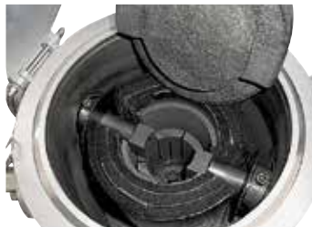
Graphite heating module
