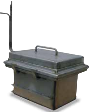
Annealing box with protective gas inlet and outlet, constructed for evacuation at ambient temperatures
