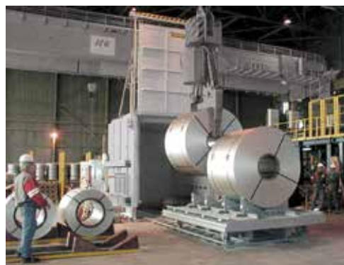
Air circulation bogie hearth furnace for heat-treating coils
