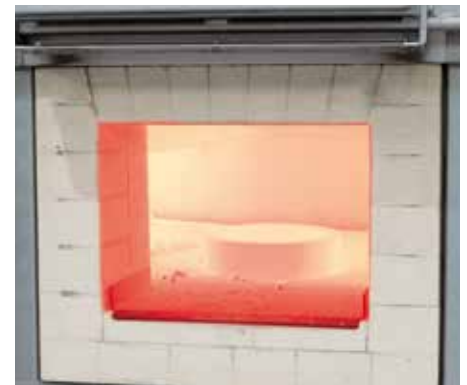
Pre-heating of steel rings for forging
