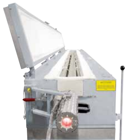
Strand annealing furnaces based on a tube furnace with a length of 6 meters
