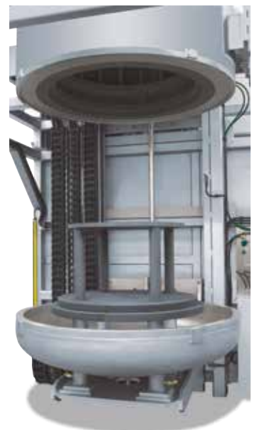
LBVHT with graphite heating chamber
