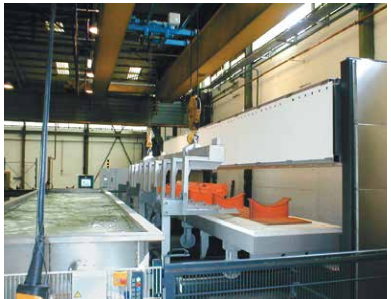
Manual tempering plant for hardening of steel rods see page 70/71
