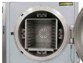
Retort with internal heating and process chamber
