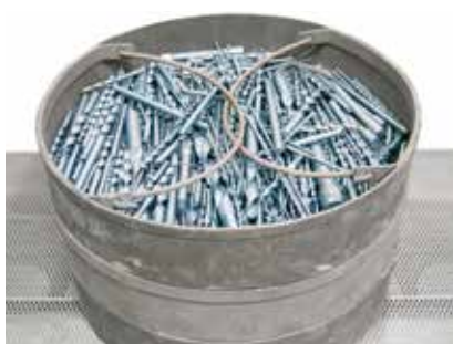
Blueing of drills in water steam atmosphere in a furnace of the NRA range see page 12
