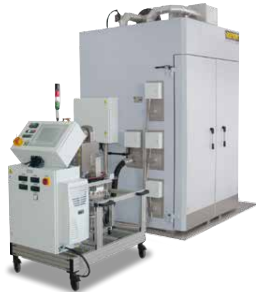
KTR 3100/S for curing of composites in vacuum bags incl. pump and necessary connections in the oven chamber
