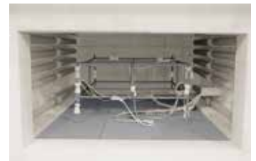
Measurement set-up in an annealing furnace
