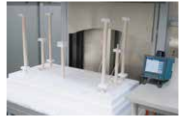
Measurement set-up in a high-temperature furnace
