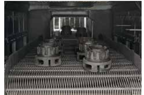
Mesh belt drive in a continuous furnace
