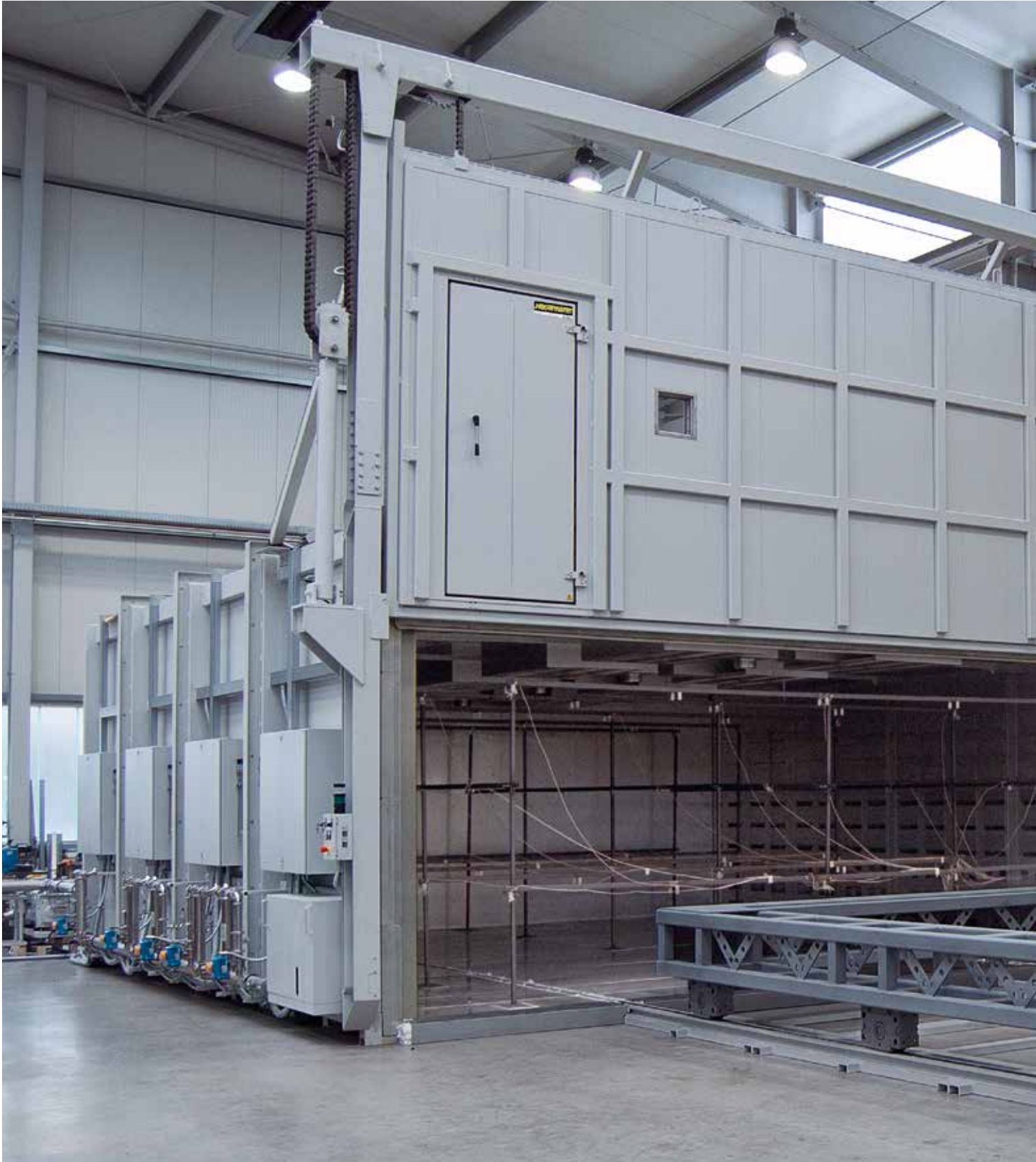
Air circulation chamber furnace N 140000/26AS for curing of composites in vacuum bags incl. pump and necessary connections in the furnace chamber
