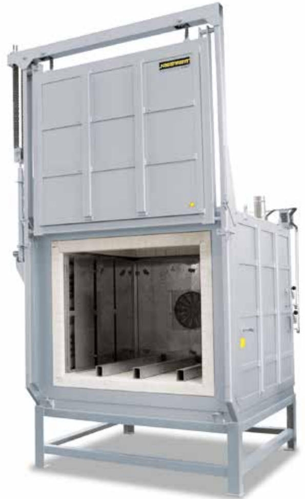
N 1500/85HA with lift door and work piece holders in the furnace
