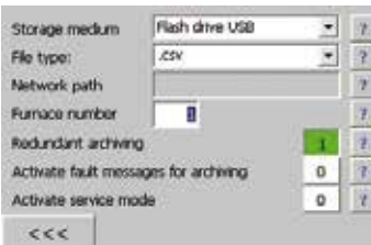
NTLog Basic for data recording of Nabertherm Controllers
