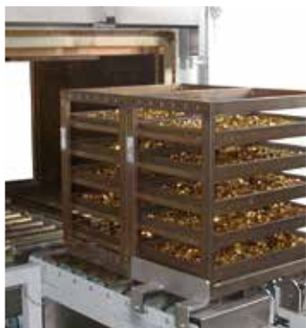
Continuous furnace for bulk materials in baskets
