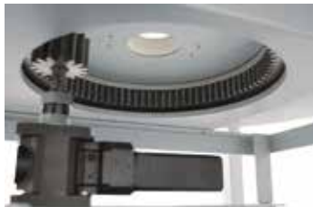
Gear rim drive under the furnace
